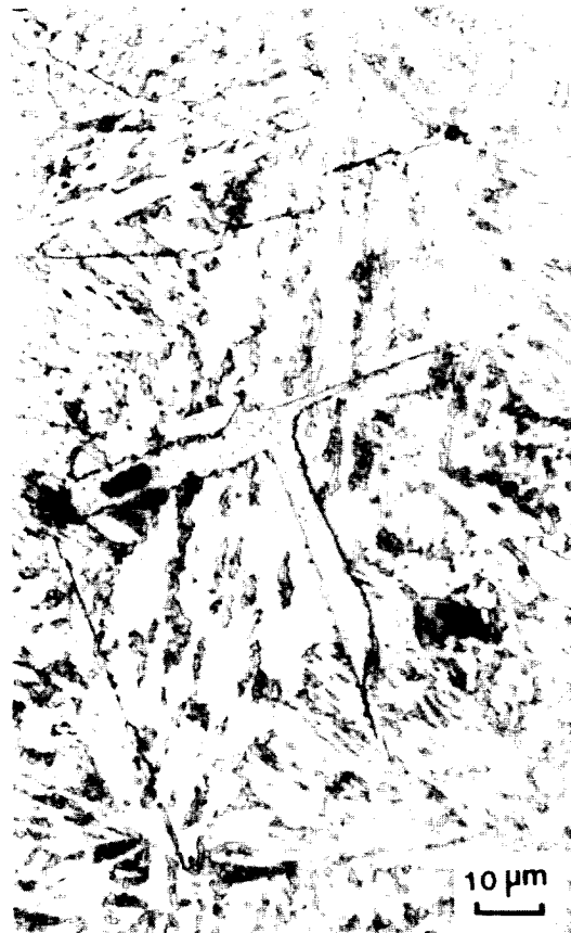
Fig. 2b. A region containing a large ferrite grain.
