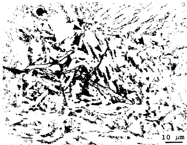
Fig. 2c. A region containing the final array of cleavage facets.
